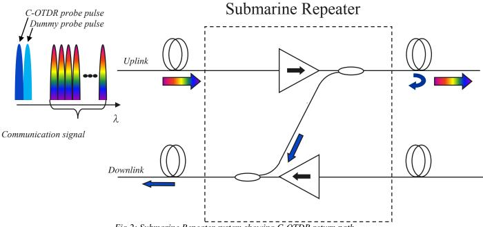
Fig 2; Submarine Repeater system showing C-OTDR return path.
