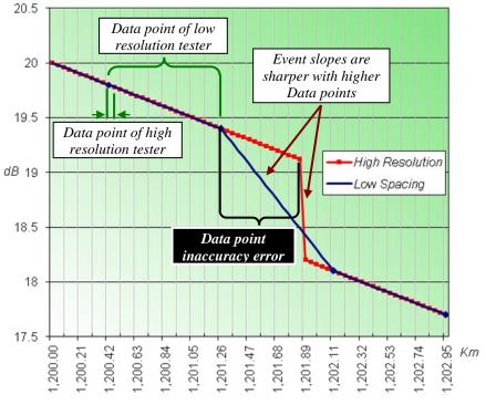
Fig 6; Data Point resolution of different C-OTDR's
